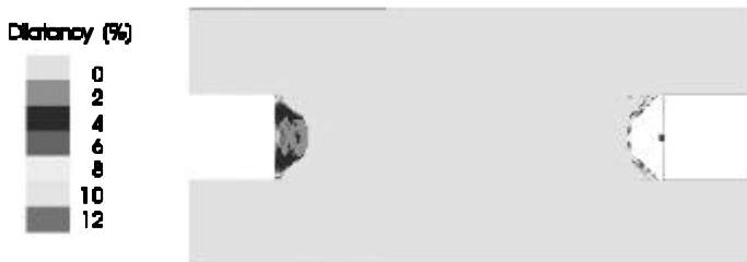
Figure 7. Dilatation development (left) and corresponding fall-out (right).
